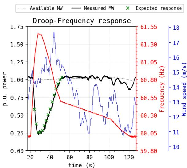
Injected frequency in red. Expected response is calculated based on frequency deviation from 60 Hz and initial power level. Data is normalized.
